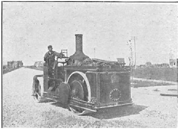
One of the principal "improvers"—steam roller for street making. Alderman Lamb's pet.
